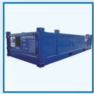
20'x8'x4' Half Height 6058 x 2438 x 1220 Gross: 13,320kg Tare: 3,320kg Payload: 10,000kg
