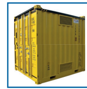
10' High Cube Dangerous 2991 x 2438 x 2896 Gross: 20,000kg Tare: 2,400kg Payload: 7,600kg
