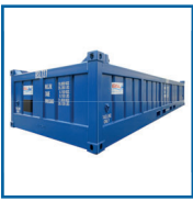
24'x8'x4'2" Half Height 7315 x 2438 x 1280 Gross: 16,000kg Tare: 4,150kg Payload: 11,850kg
