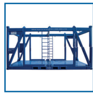
6.4m Lifting Frame 6488 x 2838 x 3285 Gross: 25,000kg Tare: 5,880kg Payload: 19,120kg
