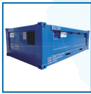
15'x8'x4'3" Half Height 4572 x 2438 x 1295 Gross: 20,000kg Tare: 2,550kg Payload: 17,450kg
