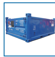
10'x8'x4' Half Height 2991 x 2438 x 1220 Gross: 7,000kg Tare: 1,400kg Payload: 5,600kg
