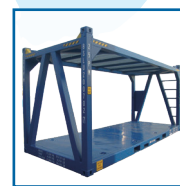
20'x8'x9'6" Lifting Frame 6058 x 2438 x 2896 Gross: 17,200kg Tare: 4,200kg Payload: 13,000kg
