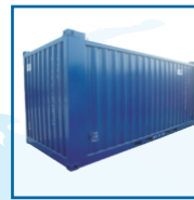
20'x8'x8'6" Dry Goods 6058 x 2438 x 2591 Gross: 20,000kg Tare: 3,850kg Payload: 16,150kg
