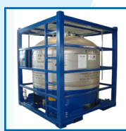
5000L Offshore Portable Tank 2300 x 2300 x 2560 Tare: 2,450kg Payload: 7,550kg
