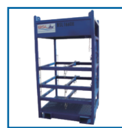
Bottle Rack 1270 x 1150 x 2285 Gross: 2,500kg Tare: 550kg Payload: 1,950kg
