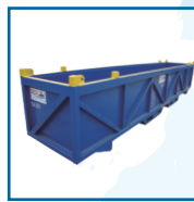
6.3m Cargo Basket 21' x 4' x 4'3" 6300 x 1200 x 1300 Gross: 13,000kg Tare: 1,900kg Payload: 11,100kg
