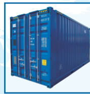
20'x8'x9'6" High Cube 6058 x 2438 x 2896 Gross: 20,000kg Tare: 4,250kg Payload: 15,750kg
