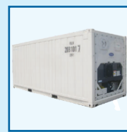
20'x8'x8'6" Reefer 6058 x 2438 x 2591 Gross: 14,200kg Tare: 4,380kg Payload: 9,820kg
