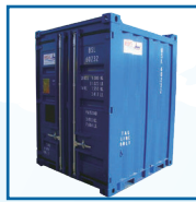
6'x6'x8' Mini 1830 x 1830 x 2438 Gross: 5,000kg Tare: 1,350kg Payload: 3,650kg
