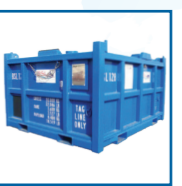
20'x8'x8'6" HSE/Spare 6058 x 2438 x 2591 Gross: 20,000kg Tare: 3,750kg Payload: 16,250kg
