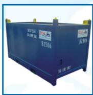
2.5m Cargo Basket 8' x 4' x 3'8" 2500 x 1220 x 1133 Gross: 7,000kg Tare: 670kg Payload: 6,330kg
