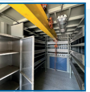
20'x8'x8'6" Workshop w/ Overhead Hoist 6058 x 2438 x 2591 Gross: 20,000kg Tare: 4,000kg Payload: 16,000kg * AC available
