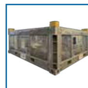
10ft Hot Dip Galvanized Subsea Basket 2991 x 2438 x 1220 Gross: 10,000kg Tare: 3,100kg Payload: 6,900kg
